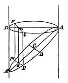
Draw a plane through AA', the transverse axis, perpendicular to the plane of the ellipse, and in this plane describe a circle on AA' as diameter. Also take the chord AD, equal to the conjugate axis, and join A'D, which is perpendicular to AD.
